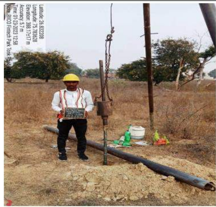
Fig: Conducting Standard Penetration Test at Site
