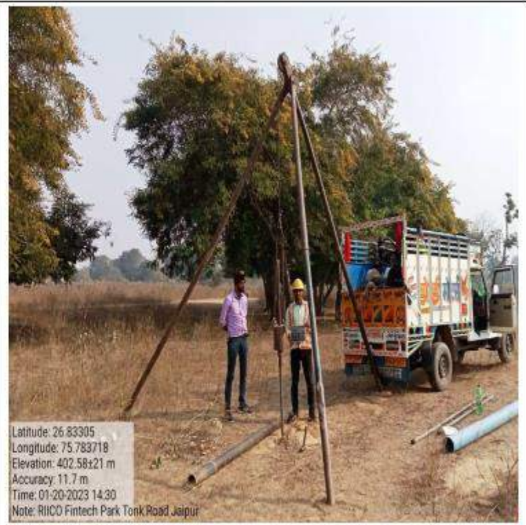
Conducting SPT Test at Site
