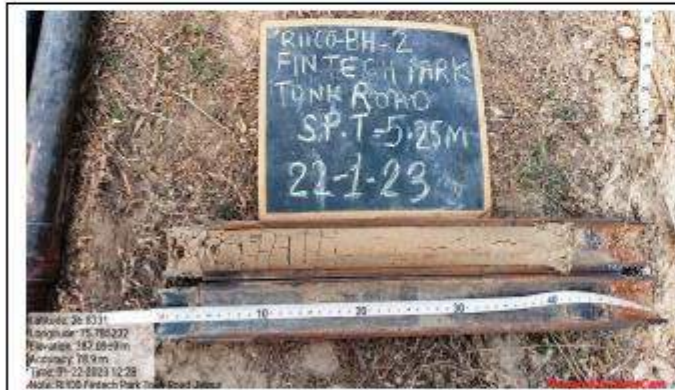
Fig: Collection of Soil Samples at Site (DS & UDS)
