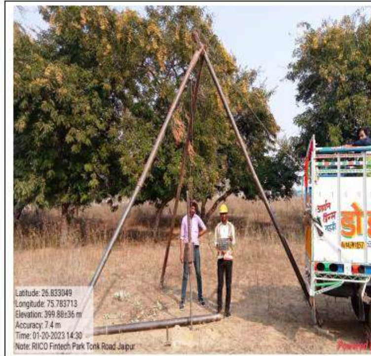
Fig: Conducting Standard Penetration Test at Site
