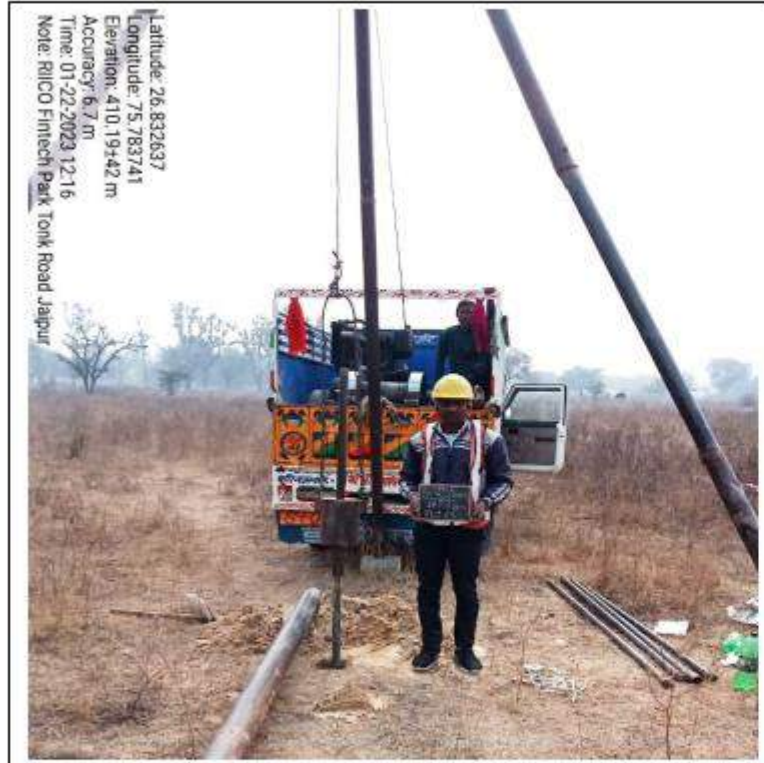
Conducting SPT Test at Site
