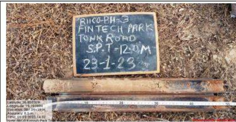
Fig: Collection of Soil Samples at Site (DS & UDS)
